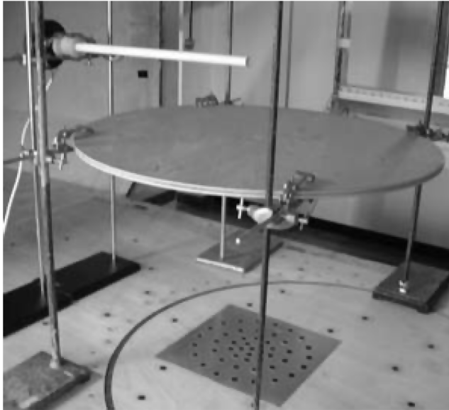
Fig. 16 Photo showing the measurement setup for sound diffraction around a disk in the Markham wind tunnel.
